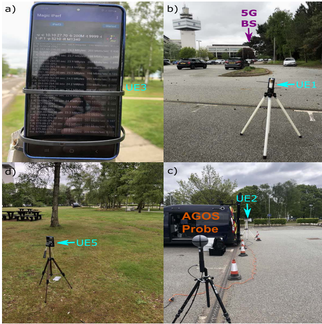
FIGURE 4. Ground view of the various equipment used in our exposure measurement setup for the commercial 5G BS: a) Samsung 5G mobile phone (UE3) with 'iPerf' application; b) view of the test site and 5G BS location from the rear of UE1 (mounted on a tripod); c) view of the test site from the left side of the AGOS probe, showing the AGOS probe and UE2 relative position; d) view of the test site from the rear of UE5.
