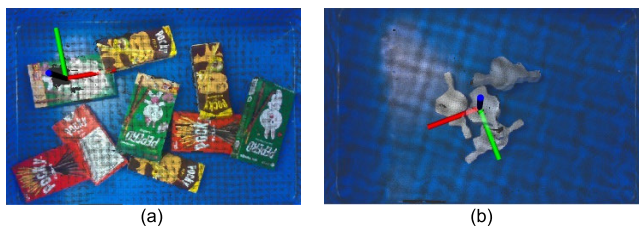
FIGURE 23. Object pose estimation results of two orientation required experiments: (a) Experiment C, and (b) Experiment D.
