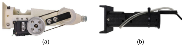
FIGURE 17. Two self-made vacuum tools used in the experiment: (a) 1-DOF vacuum tool, (b) small nozzle vacuum tool.
