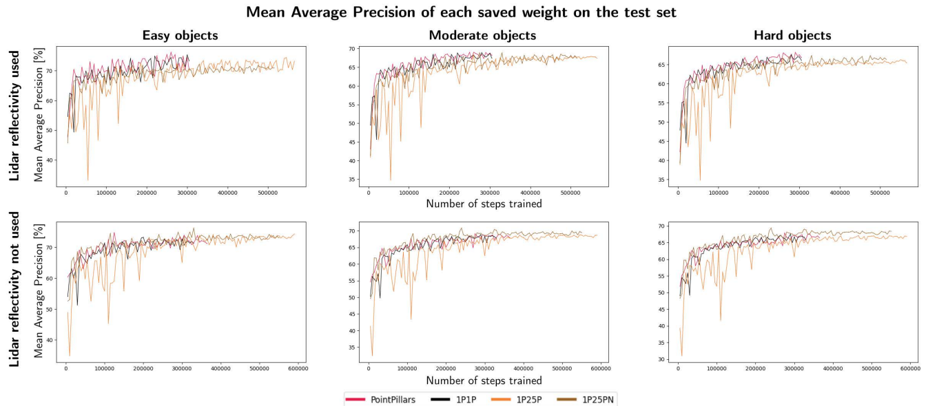
FIGURE 6. Mean Average Precision (mAP) values for each trained weights, saved during training. The 1st row reflects the results for the case when lidar reflectivity was considered, the 2nd row shows the results when lidar reflectivity was omitted. The 1st column shows the mAP values computed on the “Easy”, the 2nd column shows the mAP values for the “Moderate”, and the 3rd column shows the mAP values for “Hard” objects. These categories are defined by the KITTI benchmark site.
