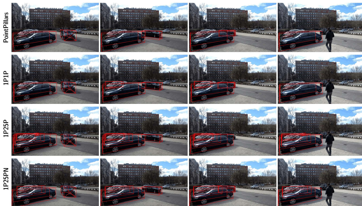
FIGURE 15. Detected vehicles in our custom dataset. The lidar reflectivity values were also included. The same four samples were given as input to the networks to compare their responses. The individual rows correspond to the responses of the original PointPillars, the 1PIP, the 1P25P and the 1P25PN networks, respectively.
