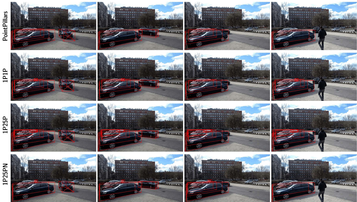
FIGURE 16. Detected vehicles in our custom dataset. Lidar reflectivity values were not used by the networks in this case. The same four samples were given to the networks to compare their responses. The individual rows correspond to the responses of the original PointPillars, the 1PIP, the 1P25P and the 1P25PN networks, respectively.
