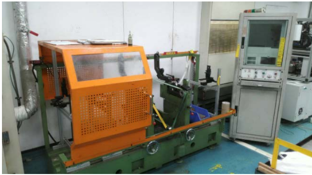
FIGURE 10. Dynamic balancing machine for IISU3EDGAN.
