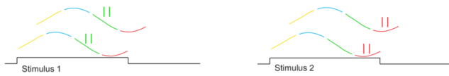
FIGURE 10. Schematic representation of phase coding. In this case, it is not possible to distinguish each stimuli through their spike count (since it is the same for both) but rather through the timing of appearance regarding the global oscillatory reference. Source: Adapted from [94].
