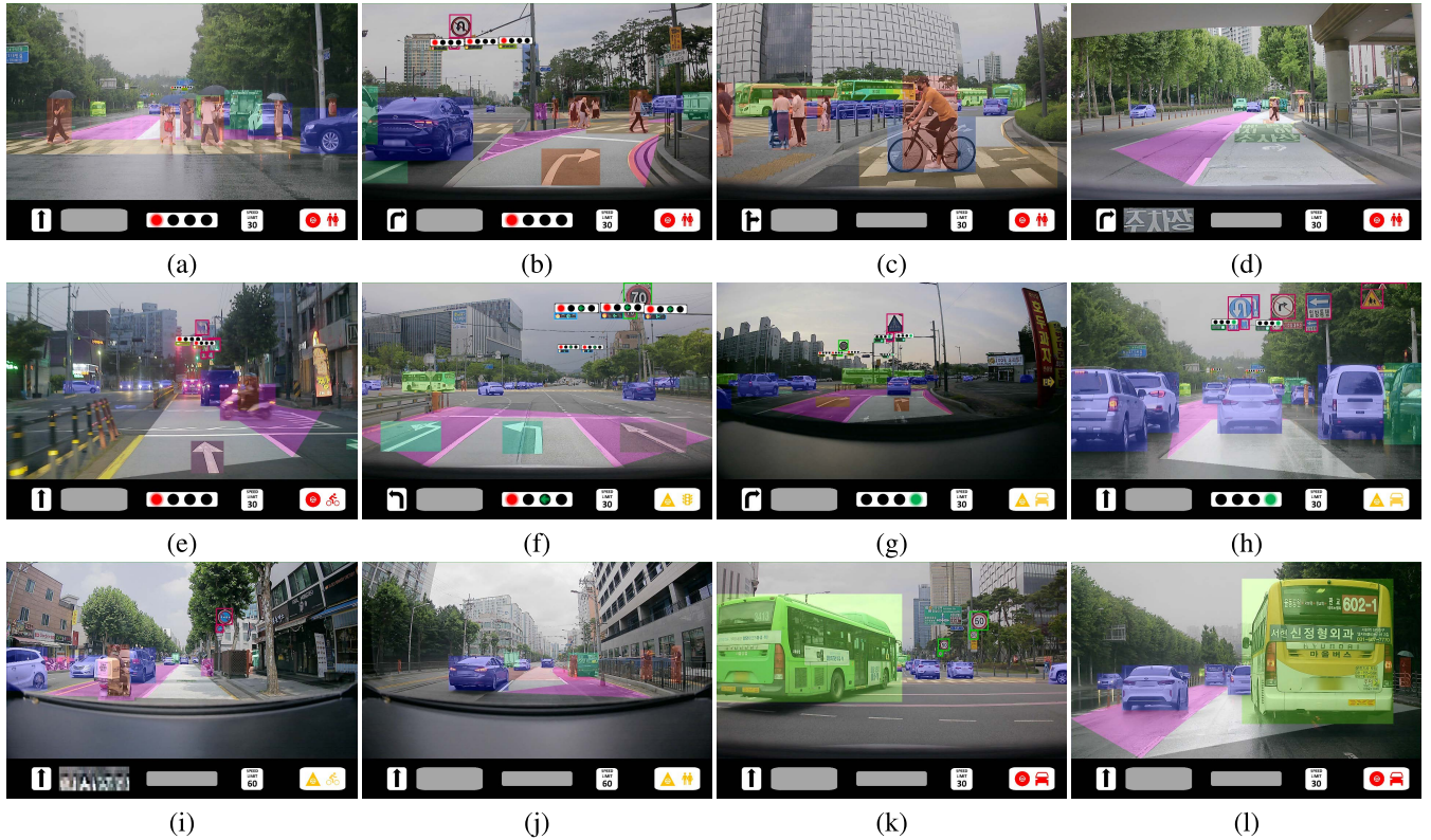
FIGURE 9. Specific cases. (a)-(c) The pedestrians are in crosswalks. (d) The pedestrian is in the ego-lane. (e) A motorbike is in front of the vehicle (f)-(h) Multiple and different types of traffic lights. (i) The motorbike is parked on the pavement. (k)-(l) The bus suddenly changes lanes.
