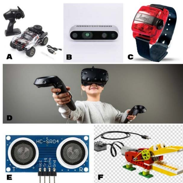
FIGURE 5. A: RC-Car; B: perceptual computing technology; C: ActiGraph GT3X; D: virtual reality headset; E: ultrasonic sensor; F: LEGO.
