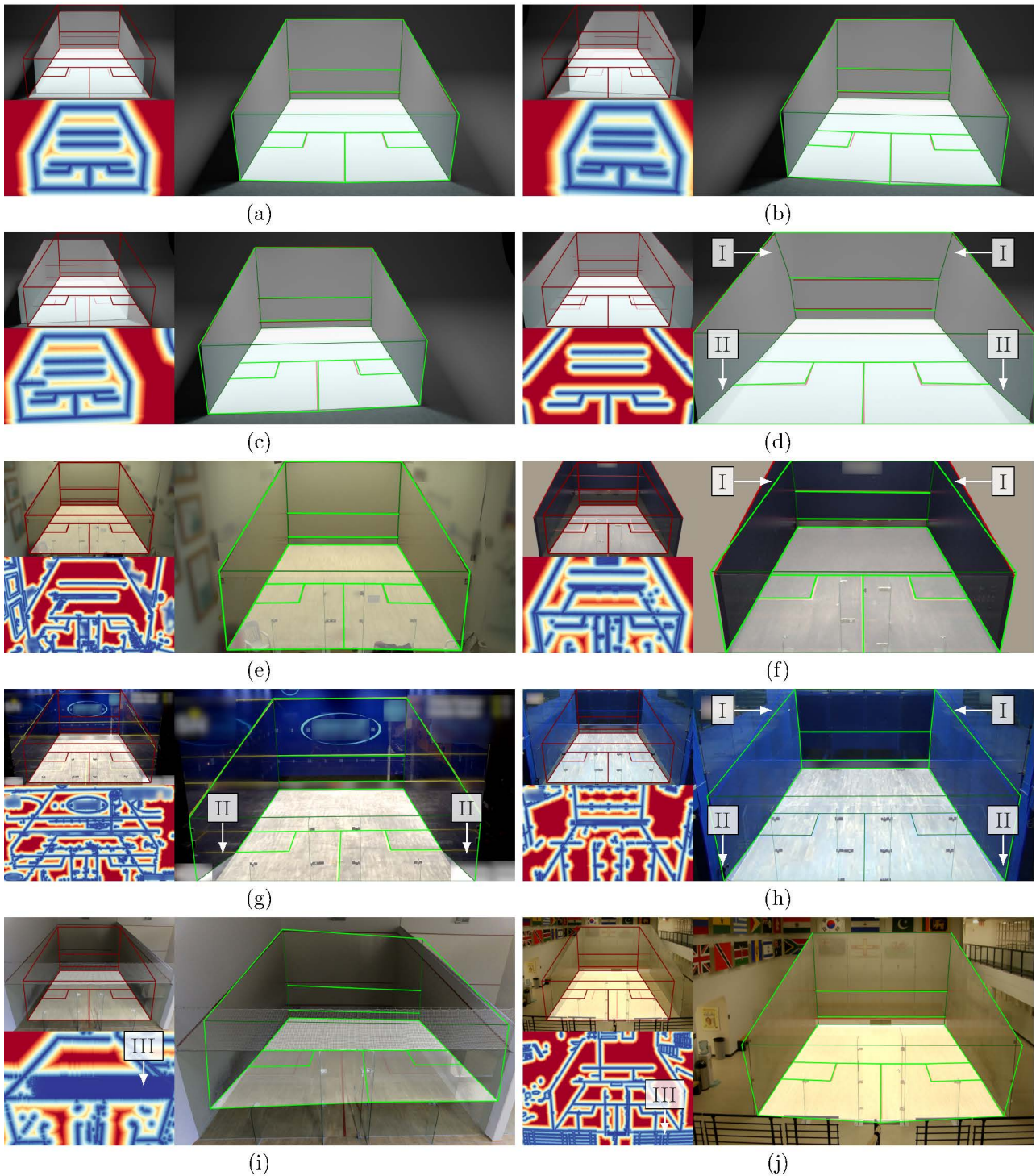
FIGURE 13. Fitness maps and geometry projections for the start and the GA optimized camera on artificial and real squash court scenarios, respectively. In (a)-(d) artificial and in (e)-(j) real world scenarios are presented. Each scenario is composed of three images. First, in the top left, geometry projection by the start camera (initial vector) is shown on top of the physical camera's captured image. Below, the fitness map obtained after edge detection is presented. Finally on the right, geometry projection by the optimized camera (result vector) is overlaid.
