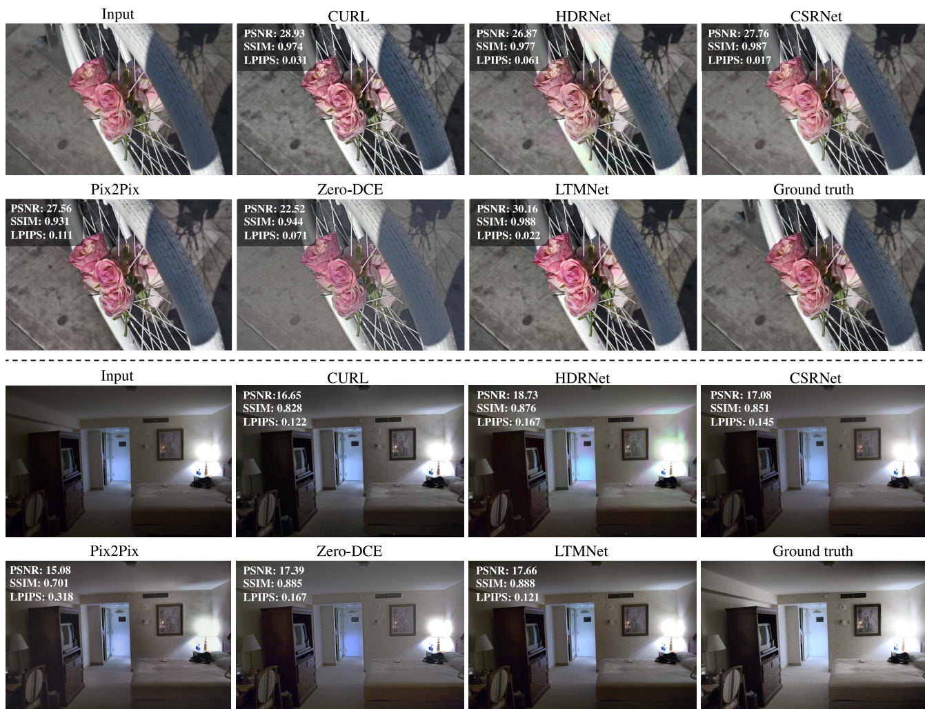
FIGURE 8. Visual comparison of our LTMNet against SOTA methods: CURL [2], HDRNet [25], CSRNet [1], Pix2Pix [64], and Zero-DCE [48], on our LTM dataset. Our LTMNet produces visually enhanced results while avoiding structural and color artifacts.
