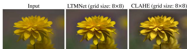
FIGURE 11. A failure example. The image contains an object in need of a significantly different transformation function from its neighbouring regions.
