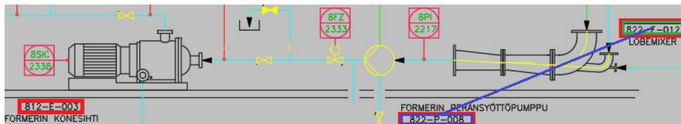
FIGURE 14. The Component_Selector application assists human experts in recognizing and selecting the desired components in the P&ID document 1 .
