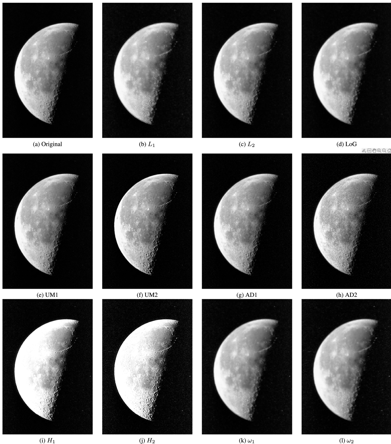
FIGURE 3. “Moon” image and its sharpened versions provided by Laplacian ( L_1 and L_2 ), LoG, high-boost ( H_1 and H_2 ), unsharp marking (UM1 and UM2), anisotropic diffusion (AD1 and AD2), and kriging-weighted Laplacian kernels ( \omega_1 and \omega_2 ).
