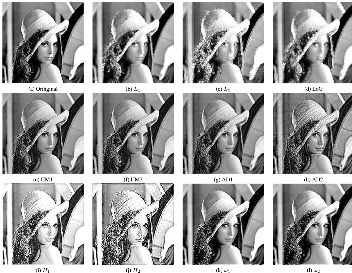
FIGURE 4. Original and sharpened images of “Lena”, using Laplacian ( L_1 and L_2 ), LoG, high-boost ( H_1 and H_2 ), unsharp masking (UM1 and UM2), anisotropic diffusion (AD1 and AD2), and kriging-weighted Laplacian kernels ( \omega_1 and \omega_2 ).
