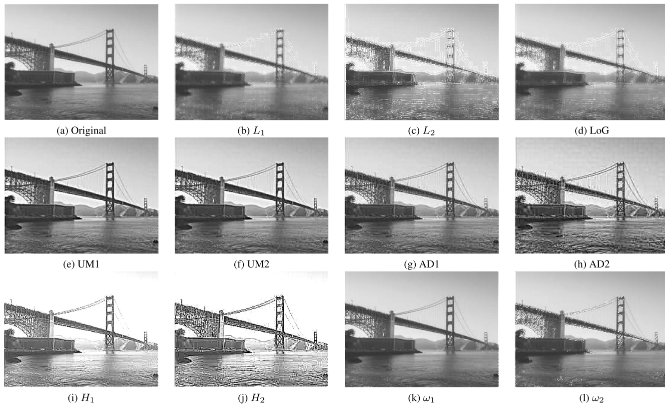
FIGURE 5. Original and sharpened images of “Bridge”, using Laplacian ( L_1 and L_2 ), LoG, high-boost ( H_1 and H_2 ), unsharp marking (UM1 and UM2), anisotropic diffusion (AD1 and AD2), and kriging-weighted Laplacian kernels ( \omega_1 and \omega_2 ).
