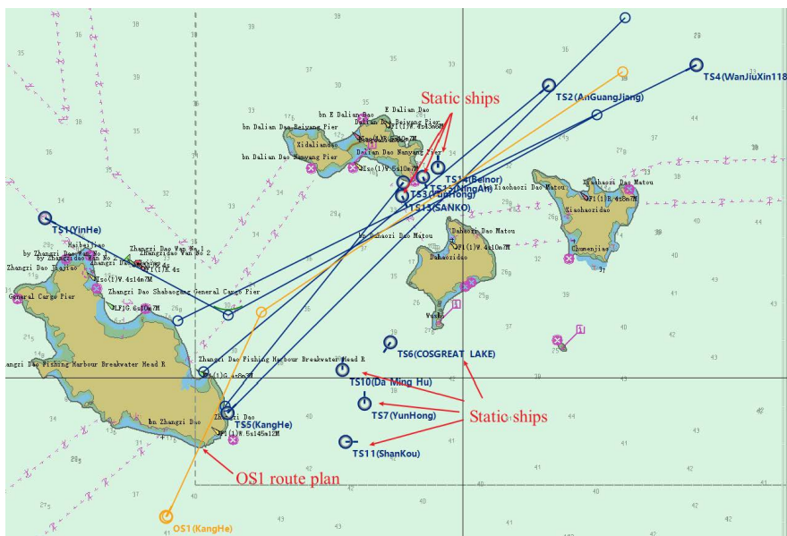
FIGURE 16. Collaborative CA and obstacle avoidance scenario including 5 moving ships and 7 static ships.
