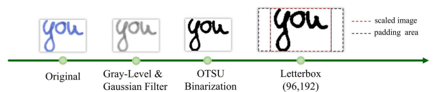
FIGURE 4. Preprocess procedure: Converted to gray-level image -> Gaussian Filtering -> OTSU Binarization -> Resizing and Padding.
