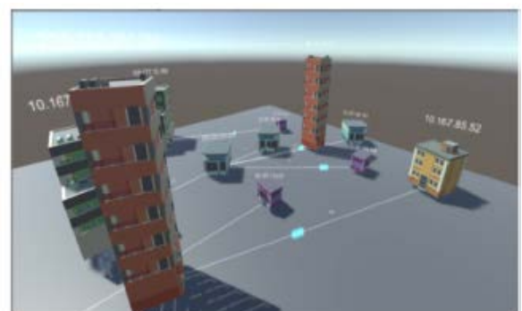
FIGURE 11. Metaphoric visualization proposed in [P1] uses the buildings and cars as metaphors to show the network activity to non-expert users. It uses the relative positioning to show the IP addresses.
