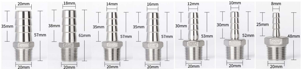
FIGURE 9. Size of 304 stainless steel hexagonal pagoda with 4 points.
