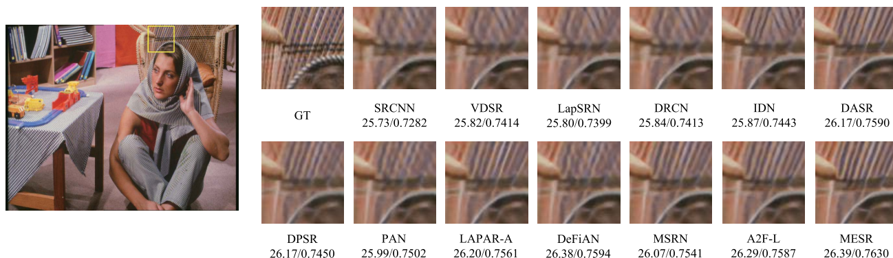
FIGURE 5. Visual comparison of super-resolution results of 'Barbara' (Set5) obtained by different SR algorithms with scaling factor \times 4 .
