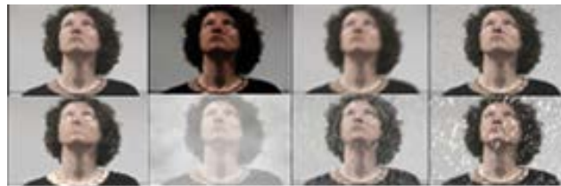
FIGURE 4. Original image and augmentation filters; snowflake, rain, contrast, fog, Gaussian noise, etc.
