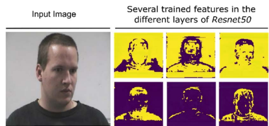
FIGURE 7. Examples of learned features by Resnet-50 feature descriptor; the output of 6 different layers are presented for illustration, e.g. from left to right; face edge, forehead, eyebrow and nose, etc.
