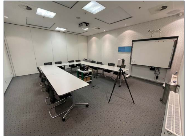
FIGURE 7. LIDAR measurement in the conference room, where LIDAR scanner is kept at position 1.
