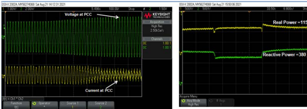
FIGURE 15. Performance of proposed FRT control scheme under HVRT mode of operation.
