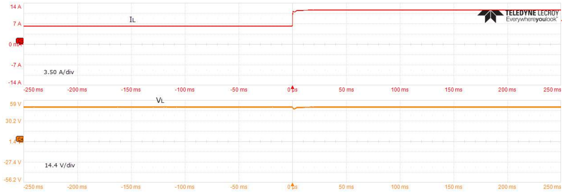
FIGURE 32. Experimental result for closed loop buck operation for 50% increase in load current.
