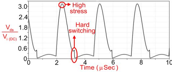
FIGURE 3. Normalized switch voltage stress of [33] with the switching frequency of  $f - 7.5\%$ .
