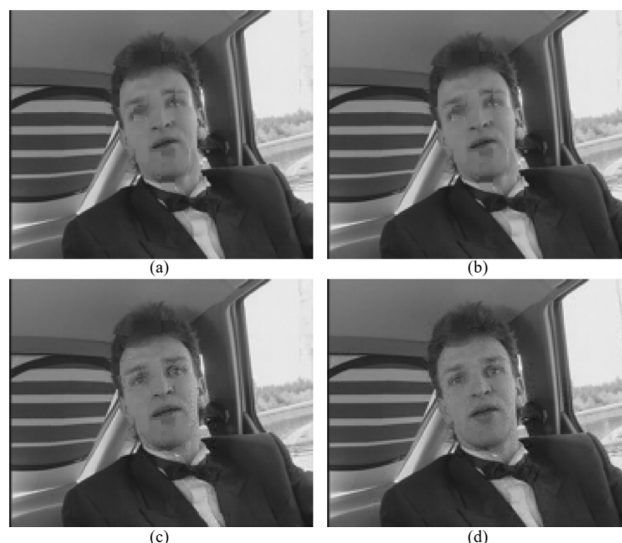
FIGURE 11. Reconstructed image (20th frame) using KMV-Cast. (a) Channel SNR = -10dB (33.42dB). (b) Channel SNR = -5dB (33.42dB). (c) Channel SNR = 0dB (37.14dB). (d) Channel SNR = 5dB (40.64dB).
