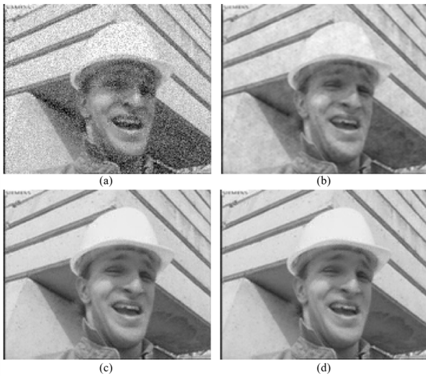
FIGURE 6. Reconstructed video quality comparisons with fairly correlated information in clouds. Channel SNR = 10dB. (a) Reconstruct 15th frame using uncoded video transmission (23.61dB). (b) Reconstruct 15th frame using SoftCast (32.73dB). (c) Reconstruct 15th frame using KMV-Cast (37.18dB). (d) Reconstruct 15th frame using proposed KMV-Cast + Wiener filter (38.36dB).
