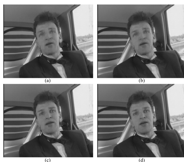
FIGURE 12. Reconstructed image (20th frame) with proposed KMV-Cast + Wiener filter. (a) Channel SNR = -10dB (34.09dB). (b) Channel SNR = -5dB (35.30dB). (c) Channel SNR = 0dB (38.51dB). (d) Channel SNR = 5dB (42.01 dB).
