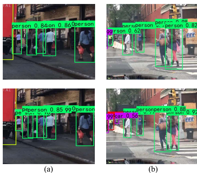
FIGURE 13. (a) Performance of YOLOv3 and the proposed detection model about the person label; (b) Performance of YOLOv3 and the proposed detection model about the person label and the rider label. The first line is the performance of YOLOv3, and the second line is the performance of the proposed detection model in (a) and (b).
