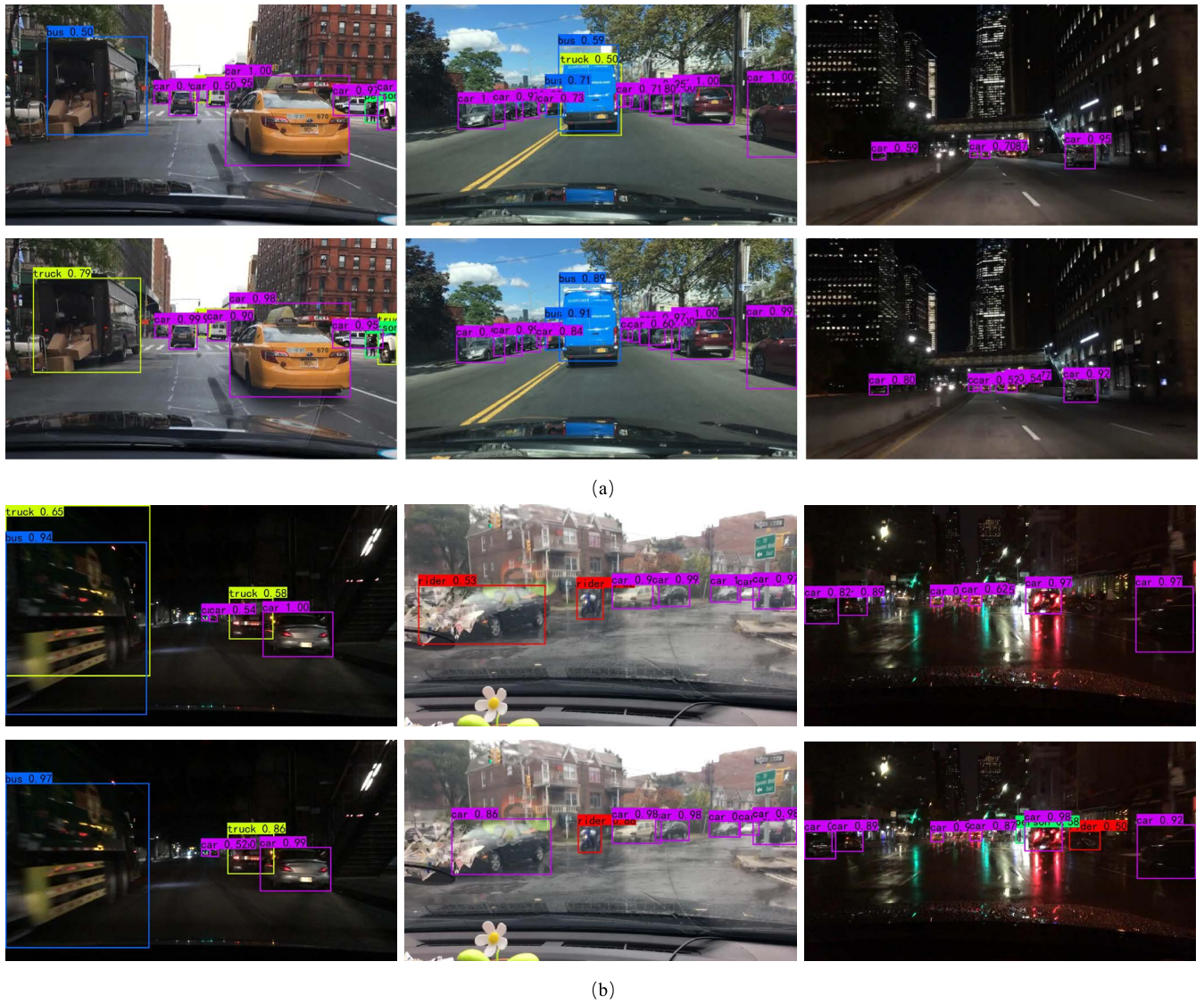
FIGURE 12. (a)Performance of YOLOv3 and the proposed detection model;(b)Performance of YOLOv3 and the proposed detection model in rainy and at night. The first line is the performance of YOLOv3, and the second line is the performance of the proposed detection model in (a)and (b).
