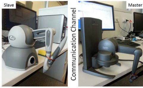
FIGURE 3. Experiment set-up for teleoperation experiment.
