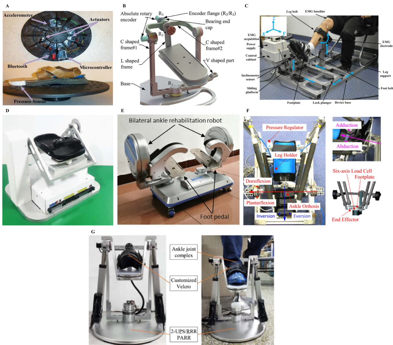
FIGURE 3. Mechanical overview of repetitive seated training robotic devices, (A) Interactive electronic wobble board system [27], (B) Parallel platform-based robotic device [28], (C) A PNF integrated robotic ankle-foot system [29], (D) An AMT [30], (E) MingKai Ankle IV (MKA-IV) rehabilitation robotic device [31], (F) Compliant Ankle Rehabilitation Robot [33], (G) Multi-modal patient compliant ankle rehabilitation system [35].
