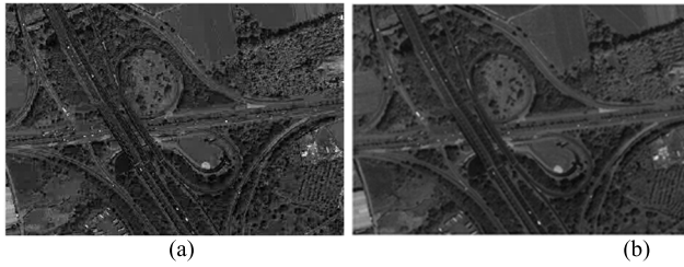
FIGURE 14. The decompressed frames of S1 with different QP and GOP configuration. (a) QP = 2/GOP = 1. (b) QP = 16/GOP = 12.
