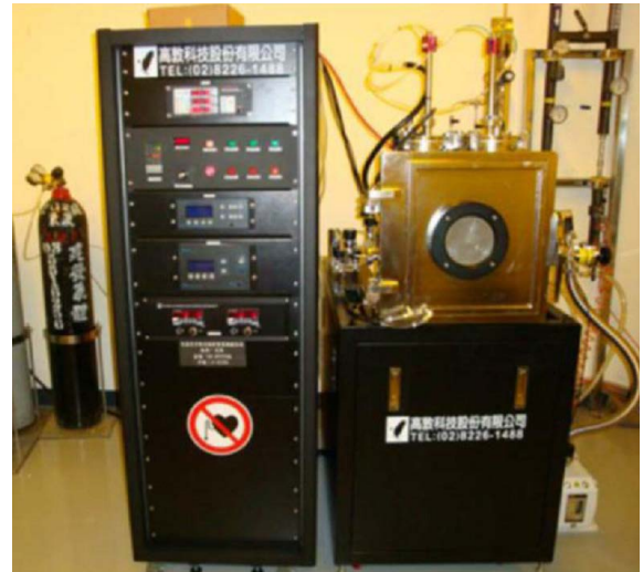
FIGURE 2. The sputter system entity graph.
