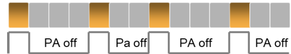
FIGURE 2. Illustration of time-domain energy saving. During symbols with no information to transmit, the PA is de-activated.
