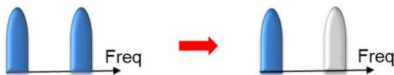
FIGURE 4. Illustration of large-scale frequency-domain energy saving, carrier shutdown. One of the two carriers is shutdown, and the related radio unit is de-activated to save energy.
