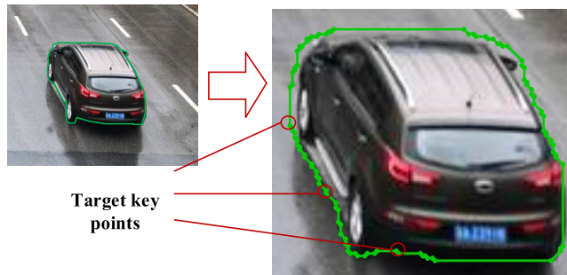
FIGURE 8. Optimization of the number of key points on the edge of the object.
