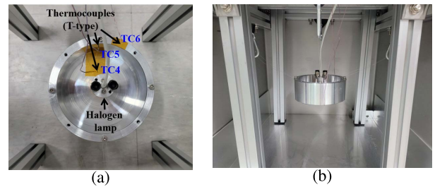
FIGURE 5. Experimental boundary conditions and sensor locations for model update process of Bottom part.
