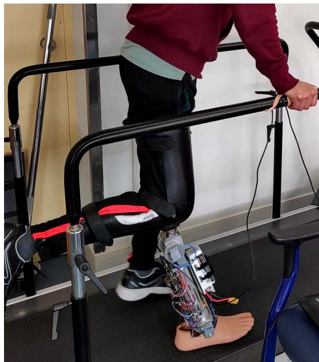
FIGURE 7. The experimental testing process for the control system of the current implementation of the prosthesis. An able-bodied adapter on a healthy subject was used for the test pilot.
