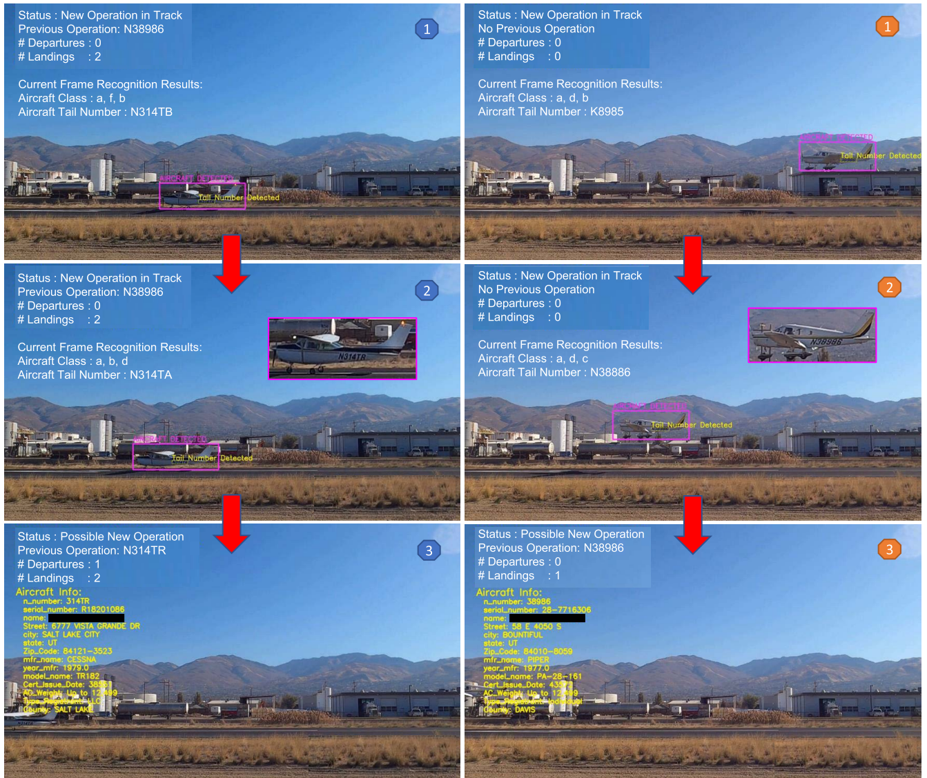
FIGURE 15. Extracted video frames from the proposed video-based identification system for two operations; aircraft identity is predicted using the two-step approach 3 once the aircraft exit the field of view.
