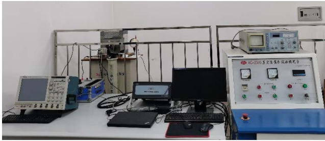
FIGURE 3. The entire experimental setup of combining detection system of electrical tree and PD.
