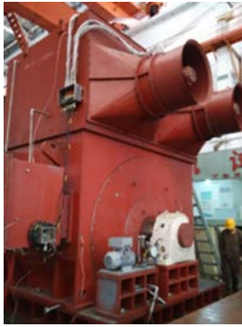
FIGURE 1. The actual prototype of positive-pressure explosion-proof motor.
