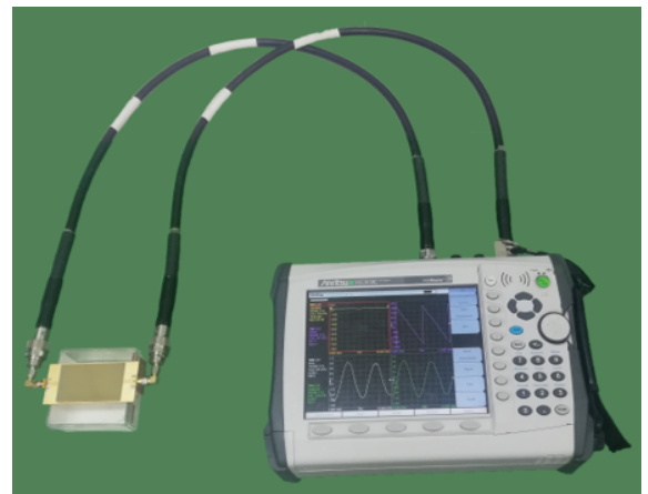
FIGURE 2. Measurement set-up: GCPW connected to a network analyzer.
