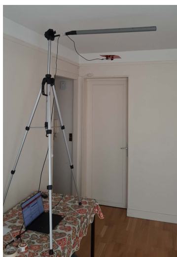
FIGURE 7. BOOSTXL-AOA angle of arrival estimation test setup.
