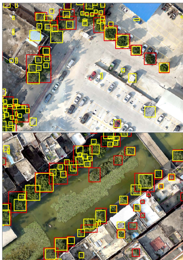
FIGURE 13. Predicted results regarding residential area, red: Faster R-CNN (Swin-T); yellow: Faster R-CNN (Resnet50).
