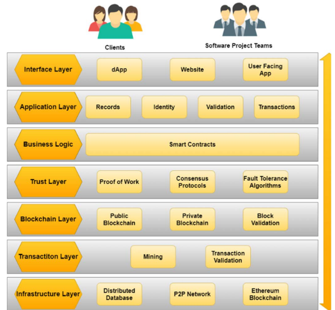
FIGURE 28. Layered Architecture for the Proposed Blockchain-Driven SRE Model.
