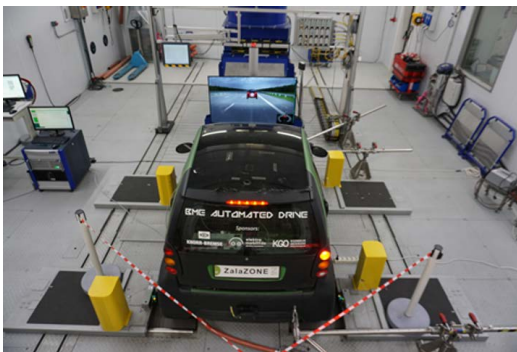
FIGURE 4. DRIVINGCUBE™ VeHIL testing environment.
