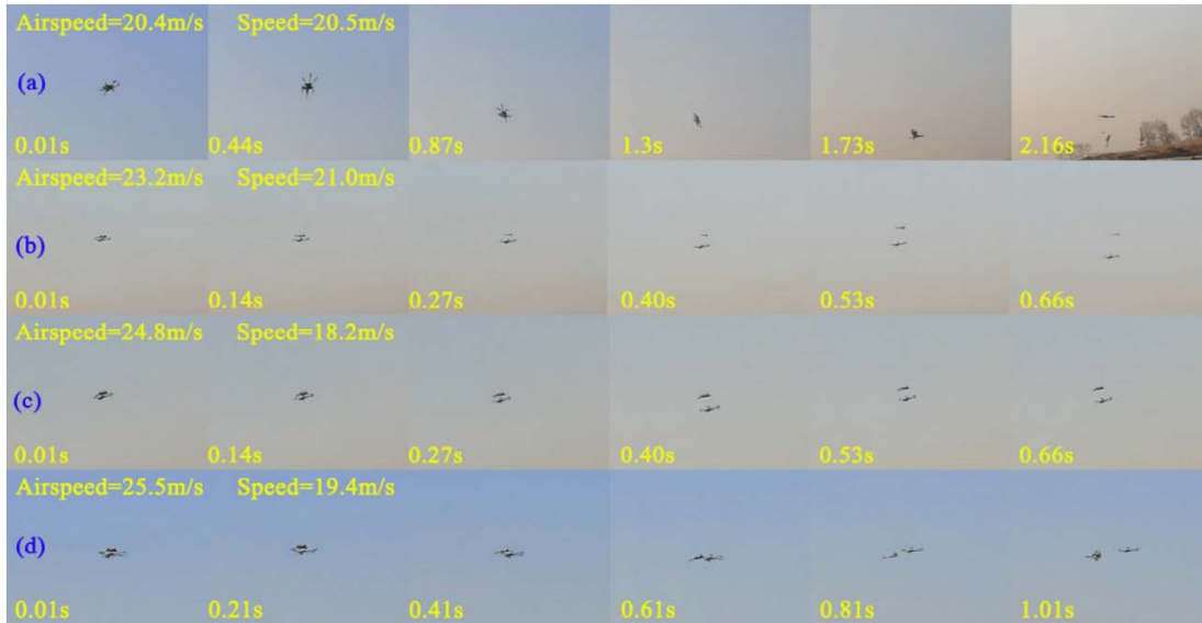
FIGURE 30. Actual separation processes of four experimental separation tests.
