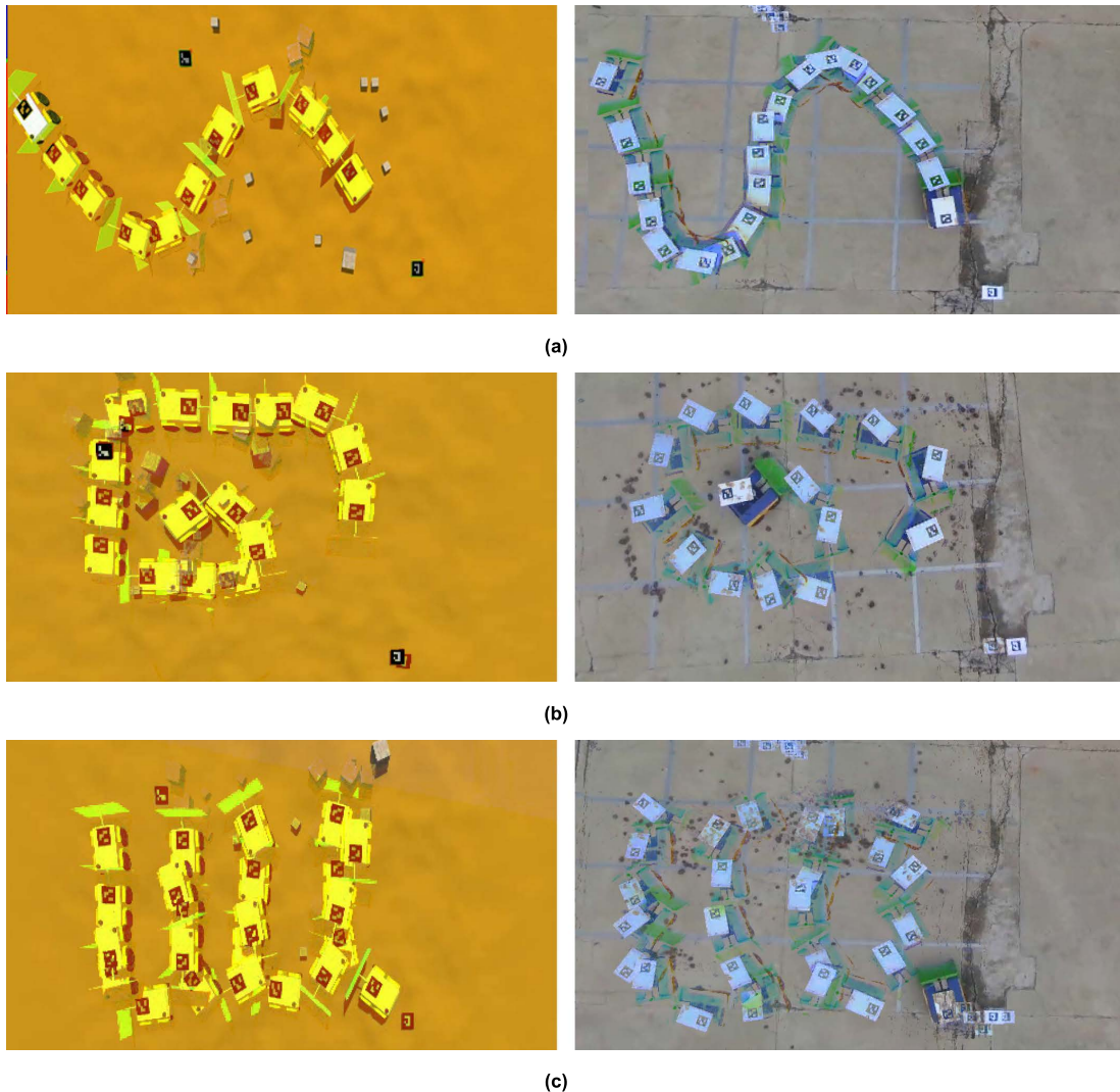
FIGURE 7. The UGV performing the (a) Slalom, (b) Spiral, and (c) Fork trajectories simulated in Gazebo (left), and the experiments (right). Both are respectively shown as top view image sequences of the simulated and actual UAV.
