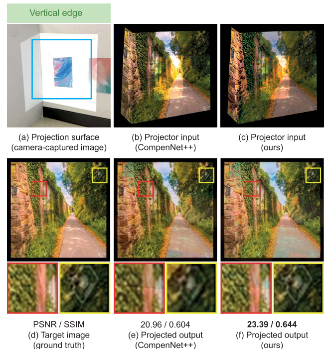
FIGURE 1. Projection mapping results of the state-of-the-art (CompenNet++) [12] and our method (ours) given a non-planar and colored projection surface. The blue-colored box (in (a)) denotes the target display area where we want to show the target (ground truth) image (d) on the surface. Both methods estimate optimal projector input images (b) and (c) for this projection mapping task by adjusting its shape and colors. Our framework optimizes the input image using differentiable rendering and produces a more accurate output image (f) than the state-of-the-art result (e).
