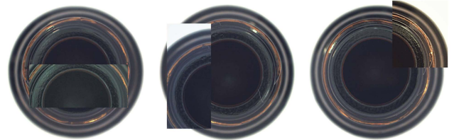
FIGURE 8. CutPaste-style processed images. An image patch is sampled from the full image, then color-jittered and pasted onto the original image.
