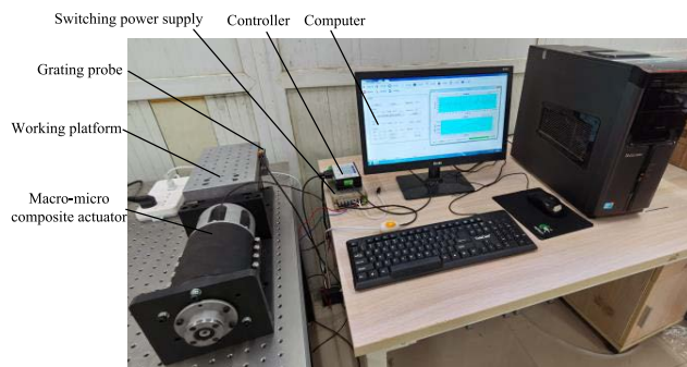
FIGURE 26. Experimental test platform for the maximum stroke and minimum positioning error.
