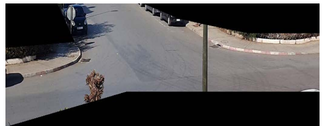
FIGURE 4. Pre-processing based on masking parking lots to eliminate some of the parked vehicles.
