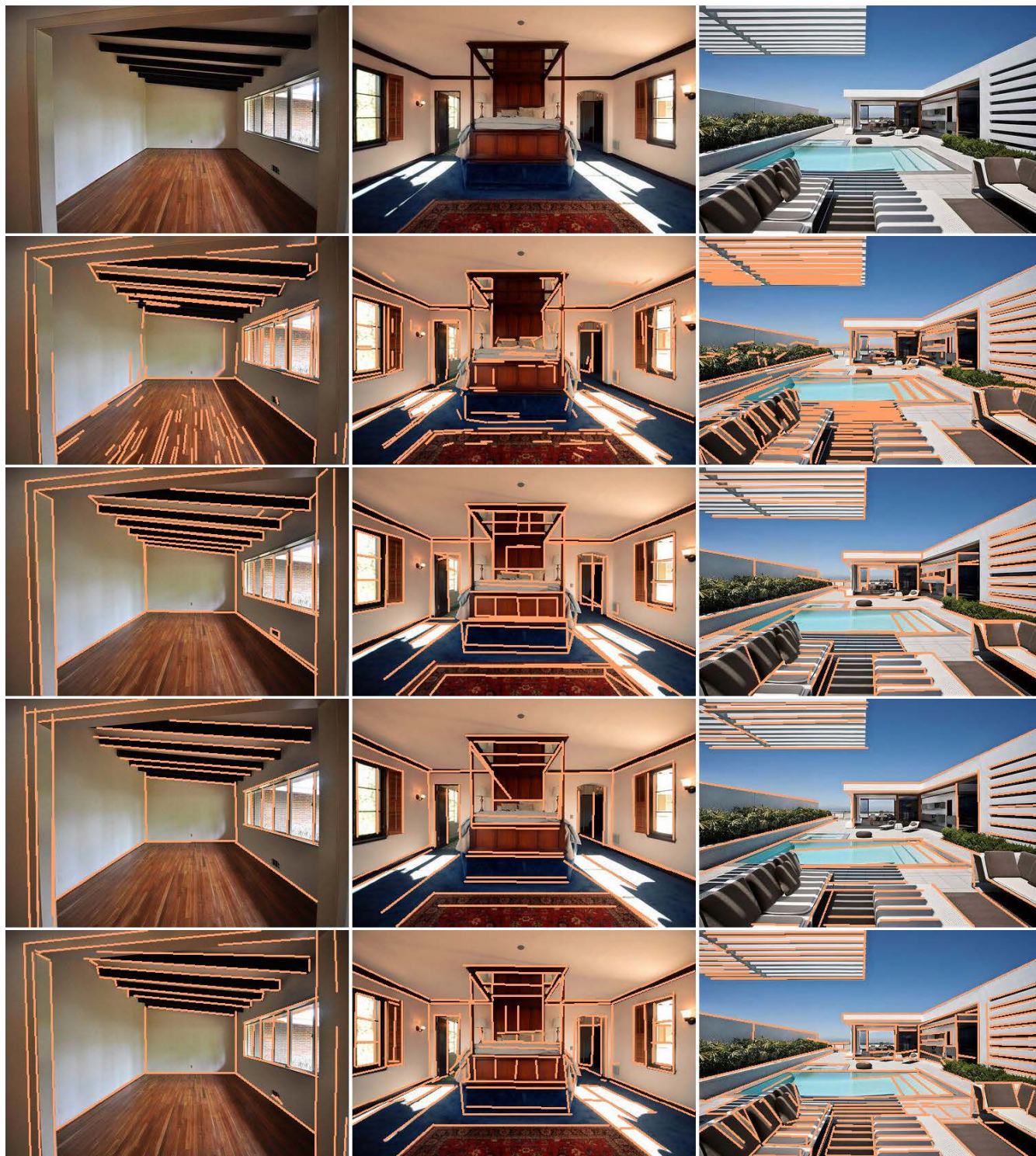
FIGURE 6. Qualitative evaluation. From left to right - images from Wireframe dataset of varying number of salient line segments. From top to bottom - original image, detection results from LSD [8], the model-based detector; HAWP [15], the most accurate CNN-based detector; M-LSD-tiny [20], the fastest CNN-based detector except for the proposed one; the proposed LSDNet. Best viewed in color and zoom-in.
