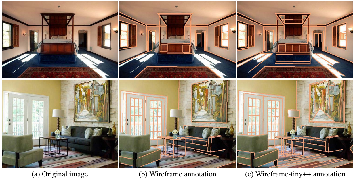
FIGURE 4. An image from Wireframe dataset (a) and two versions of its annotation - original (b) and proposed (c). Best viewed in color and zoom-in.
