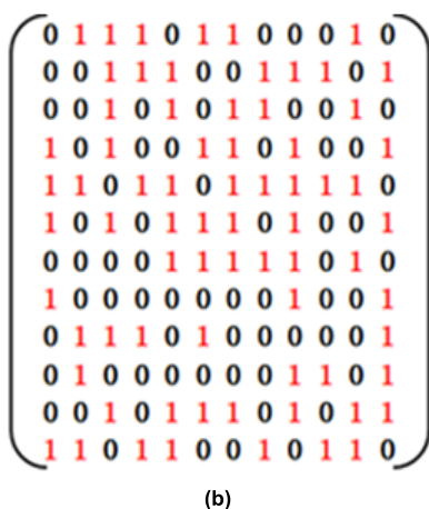
FIGURE 7. Optimization of lattice distribution by GA: (a) Program flow chart. (b) Lattice sequence matrix A*.
