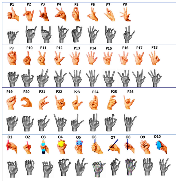
FIGURE 8. Reproduction of static postures. Quaternions converted to Euler angles and reproduced using a hand model in SOLIDWORKS. Row 1- Bharatanatyam Postures (P1 to P8), Row 2- ASL numbers (P9-P18), Row 3- ASL letters (P19-P26), Row 4- Objects to be grasped (O1-O10).
