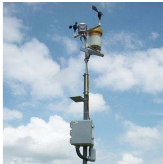
FIGURE 18. Satellite Internet-based data acquisition and control [157]. The satellite Internet telemetry system includes a data transmitter and a rechargeable battery, as well as a ground-to-satellite antenna and mounting hardware.
