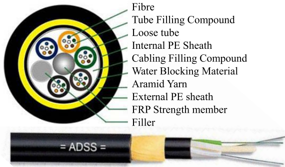
FIGURE 12. Cross section of ADSS cable [97].
