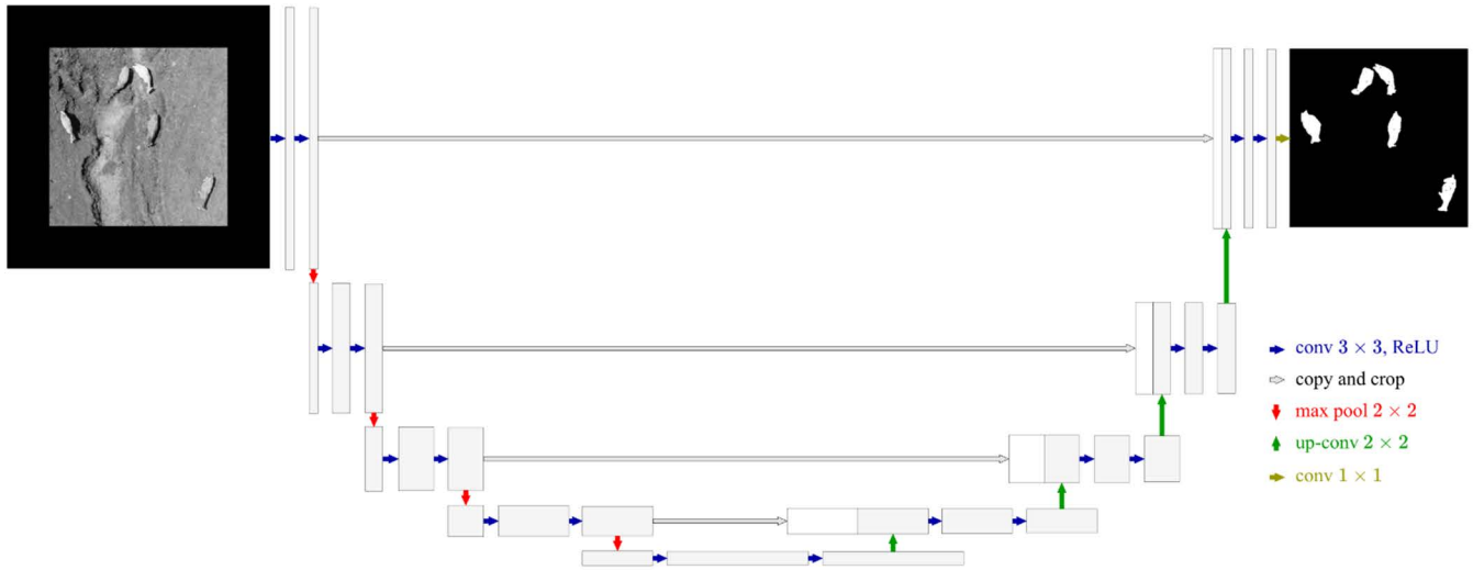
FIGURE 4. U-Net architecture for livestock segmentation (Adapted from [63]. Input image taken from [49]).
